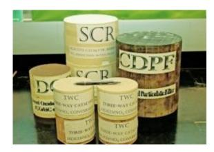
Porous ceramic bricks (monoliths) coated with precious metals and other materials lie at the heart of catalytic converter technology.  $N_2$ ,  $CO_2$  NO,  $NO_2$ NO<sub>x</sub>, NH<sub>3</sub>  $O_2$ , H<sub>2</sub>O
