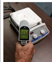
Hot plate temperature running away in the OFF position
