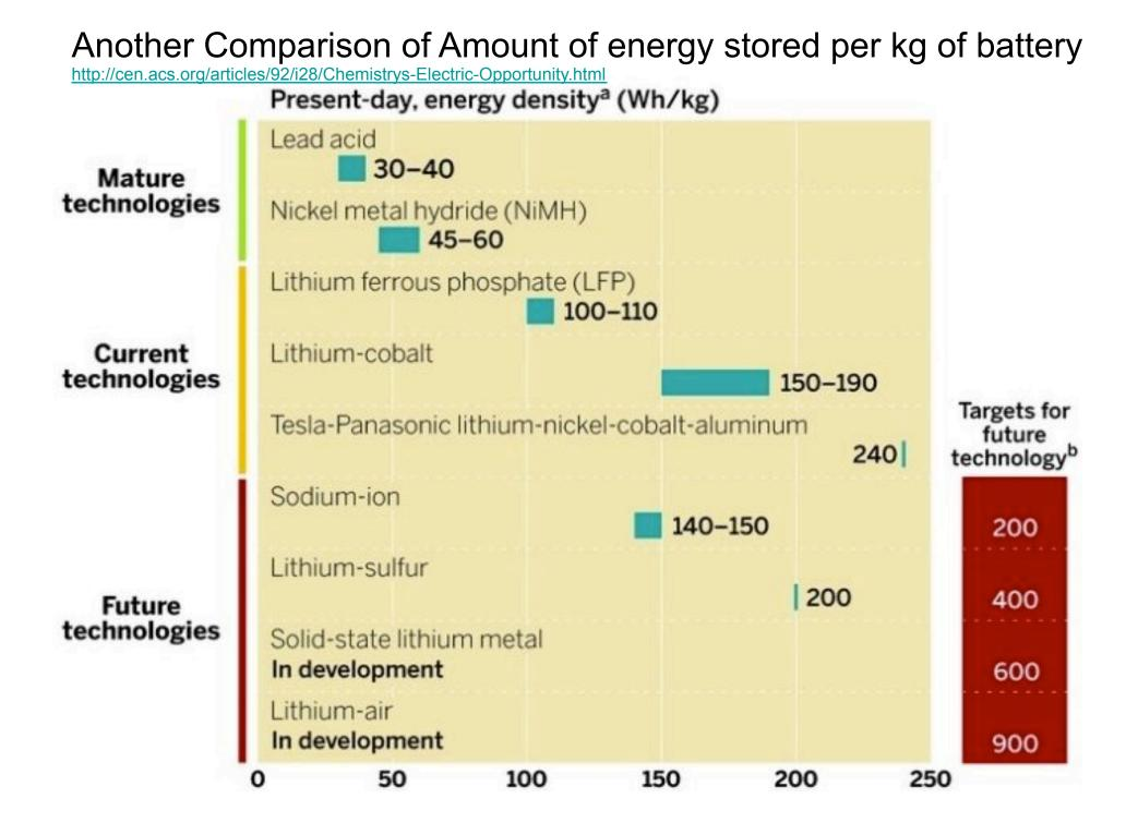
http://cen.acs.org/articles/91/i49/Researchers-Design-Lithium-Sulfur-Batteries.html Lithium-Sulfur Batteries theoretically could store *FOUR TIMES* as much energy as conventional lithium-ion batteries.
