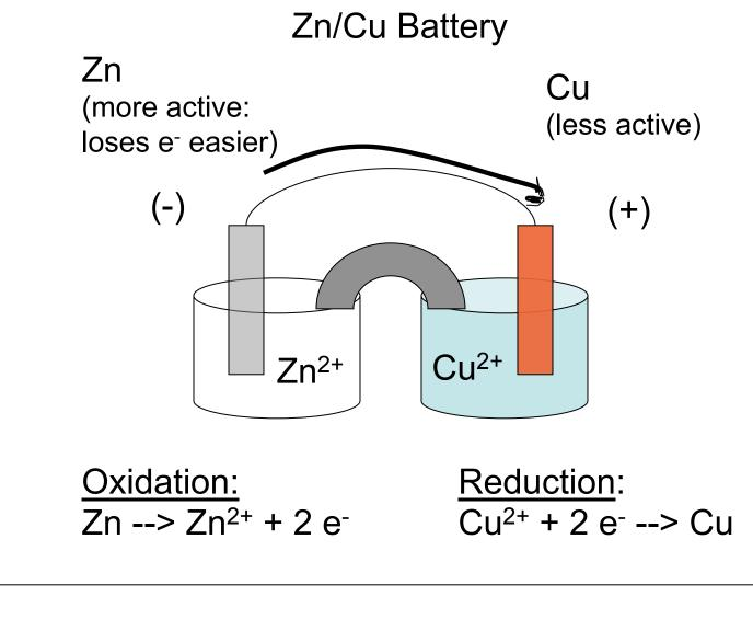
Overall cell reaction: Zn + Cu<sup>2+</sup> --> Zn<sup>2+</sup> + Cu
